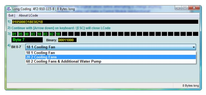
Click on each of the Byte numbers in row 3) and you'll see the selectable options below. Check or Un-check the boxes for the desired results. Example: "Adaptive Cruise Control (ACC) installed". In some cases, there will be a drop-down menu that assigns the correct bits for more complex operations.
