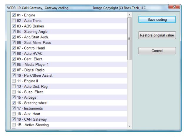
**Long Coding.** This function is needed to Code some control modules in the newest cars which use CAN for diagnostics. Due to the complexity of Long Coding strings (up to 255 bytes of hexadecimal data) we've accommodated (and urge) the use of Copy & Paste in this function and usage of the Long Coding Helper.
