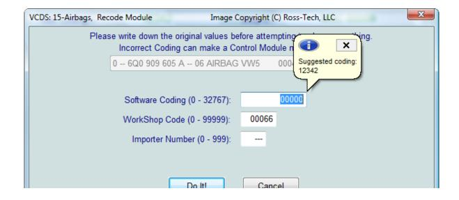
In cases where VCDS would offer Airbag module coding suggestions but cannot determine the Index automatically, VCDS gives you the ability to manually enter an Index (found on the Airbag controller sticker or work order) to get the suggested coding.
